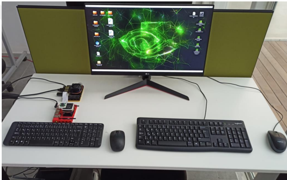
Figure 4.1 Hardware setup that contains Ubuntu 18.04 desktop computer and 2 Jetson Nano computers for simulation
