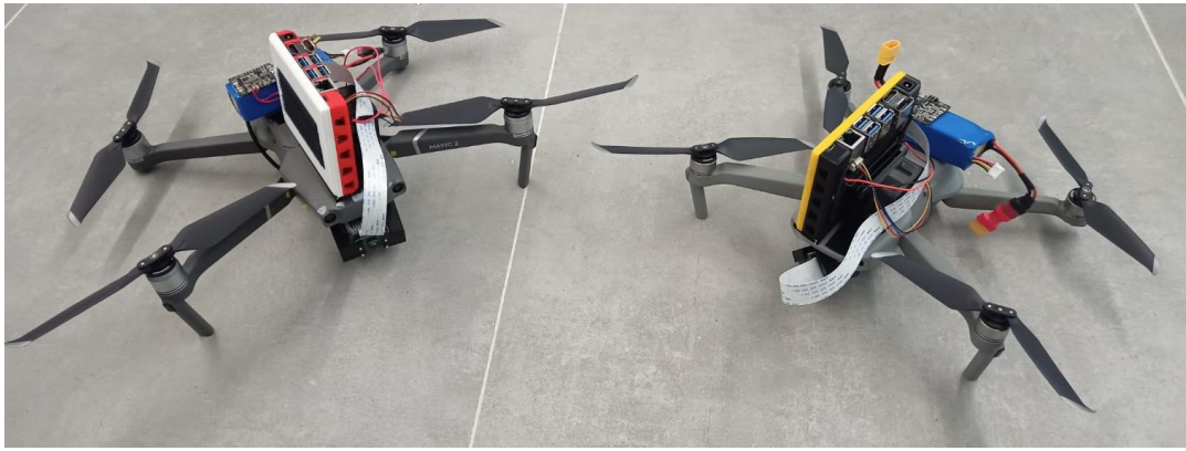
Figure 5.2 DJI “Mavic 2” and “Air 2” drones that were modified for experiment purposes.
