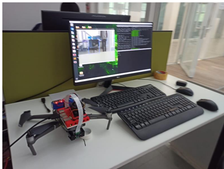
Figure 5.3 Image shows each component that was added to DJI drones
