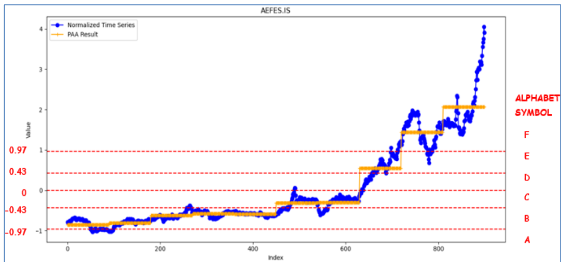
Figure 3.2 The Example of Piecewise Aggregate Approximation of AEFES For Number Segment=10 and Alphabet Size=6
