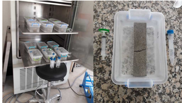
Figure 1. Experimental Setup for Nutrient Leaching Tests.
