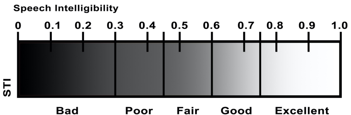
Figure 2.2.2.5.1 Results of various tests between STI and intelligibility values.
