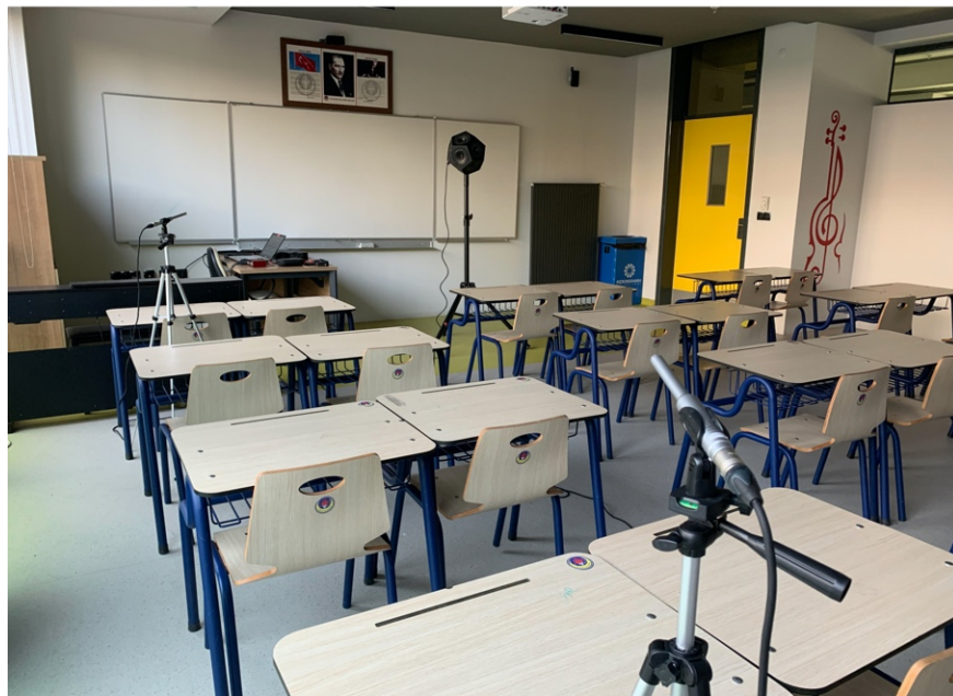
Figure 3.1.2.2 Measurement studies of the room acoustic parameters in music classrooms
