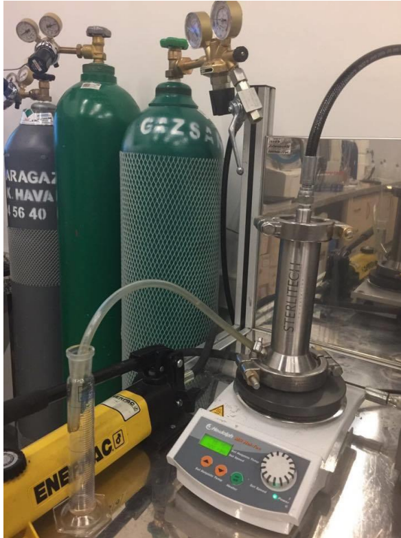
Figure 3.6. Dead-end filtration set-up
