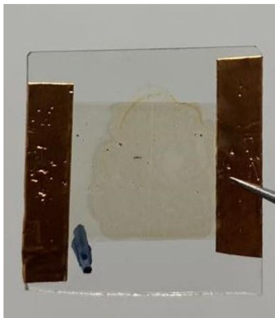
Figure 6.2 The photo of the proposed fabrication procedure to obtain metal-semiconductor-metal quantum dot photodetectors.
