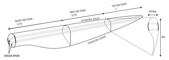
Figure 2. Dimensions of a sample 61.5 m Wind Turbine Blade from Ref. [9].
