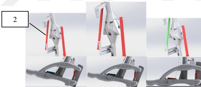
Figure 3.1.2.3 Weight acceptance mechanism and elastic element
