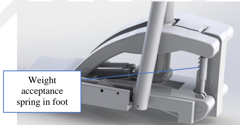
Figure 4.1.4.1 Weight acceptance spring in catapult mechanism
