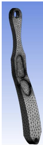
Figure 5.1.6.16 Mesh of the modified connection part.
