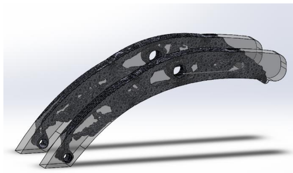
Figure 5.1.3.11 Matching the modified and raw parts
