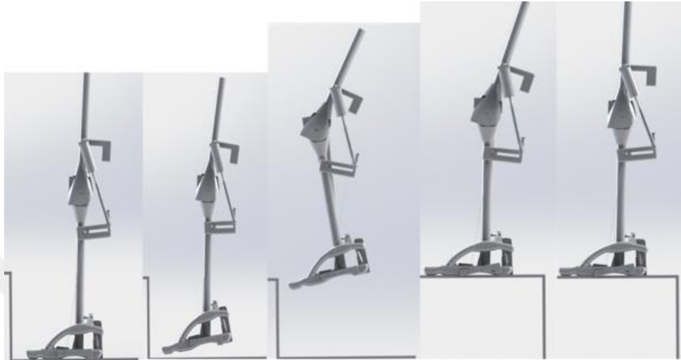
Figure 3.1.4.2 Stair climbing function of conceptual design
