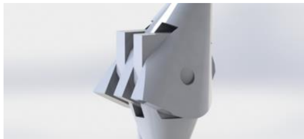
Figure 3.1.6.1 CAD design of knee
