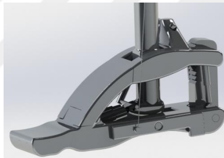
Figure 3.2.1.3 CAD design of foot-ankle compartment
