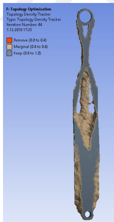
Figure 5.1.6.14 Topology optimization of the modified connection part.
