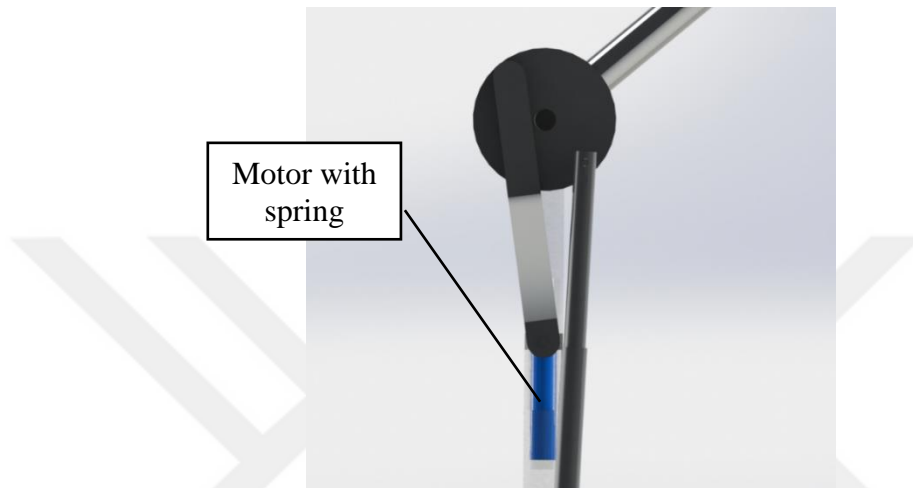
Figure 4.1.3.1 Stair ascending actuator and elastic element
