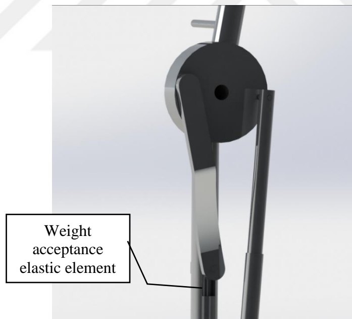
Figure 4.1.1.1 Weight acceptance elastic element
