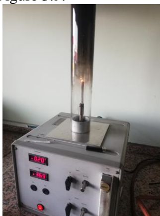
Figure 3.9 Limiting oxygen index unit in Hes Kablo
