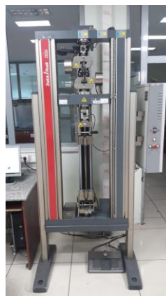
Figure 3.10 Zwick/Roell tensile test device in Hes Kablo
