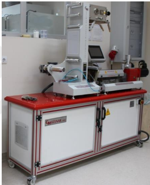
Figure 3.3 ERNAM Gülnar brand twin screw extruder
