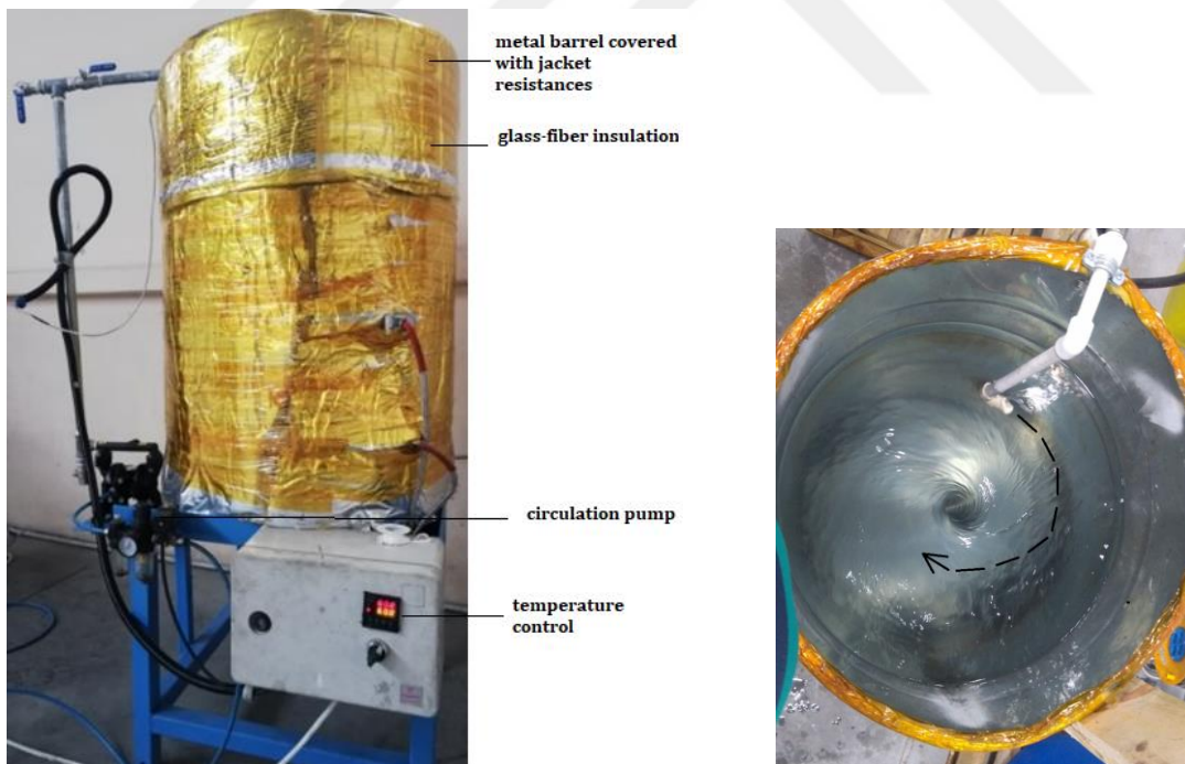
Figure 3.2 Factory-scale nanoparticle synthesis set-up
