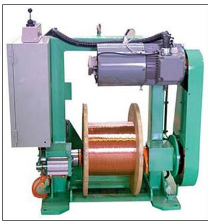
Figure 2.14 Motor driven pay-off [25]
