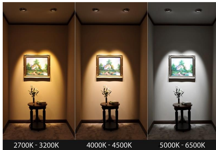
Figure 1.5.3 The effect of CCT change on vision [30]
