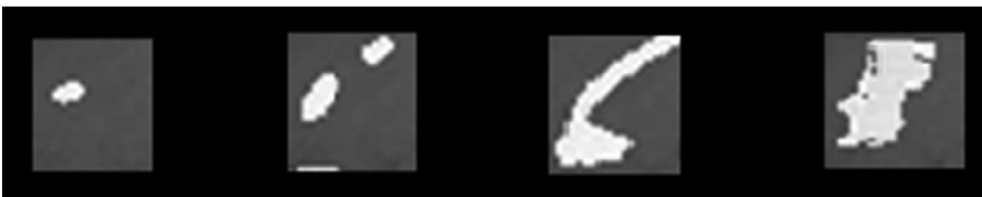
FIGURE 3 Four different size “real” reflections added on the tiles corresponding to the reflections covering 2%, 10%, 20%, and 30% of the pixels in each tile ( 32 \times 32 pixels)
